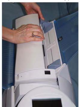
2. Squeeze the plastic clamps that hold the feed module in place and lift the feed module out of position.
